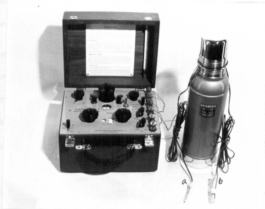
Fig.5 Thermocouple and thermocouple potentiometer set up for measuring the rectal and skin temperature.
