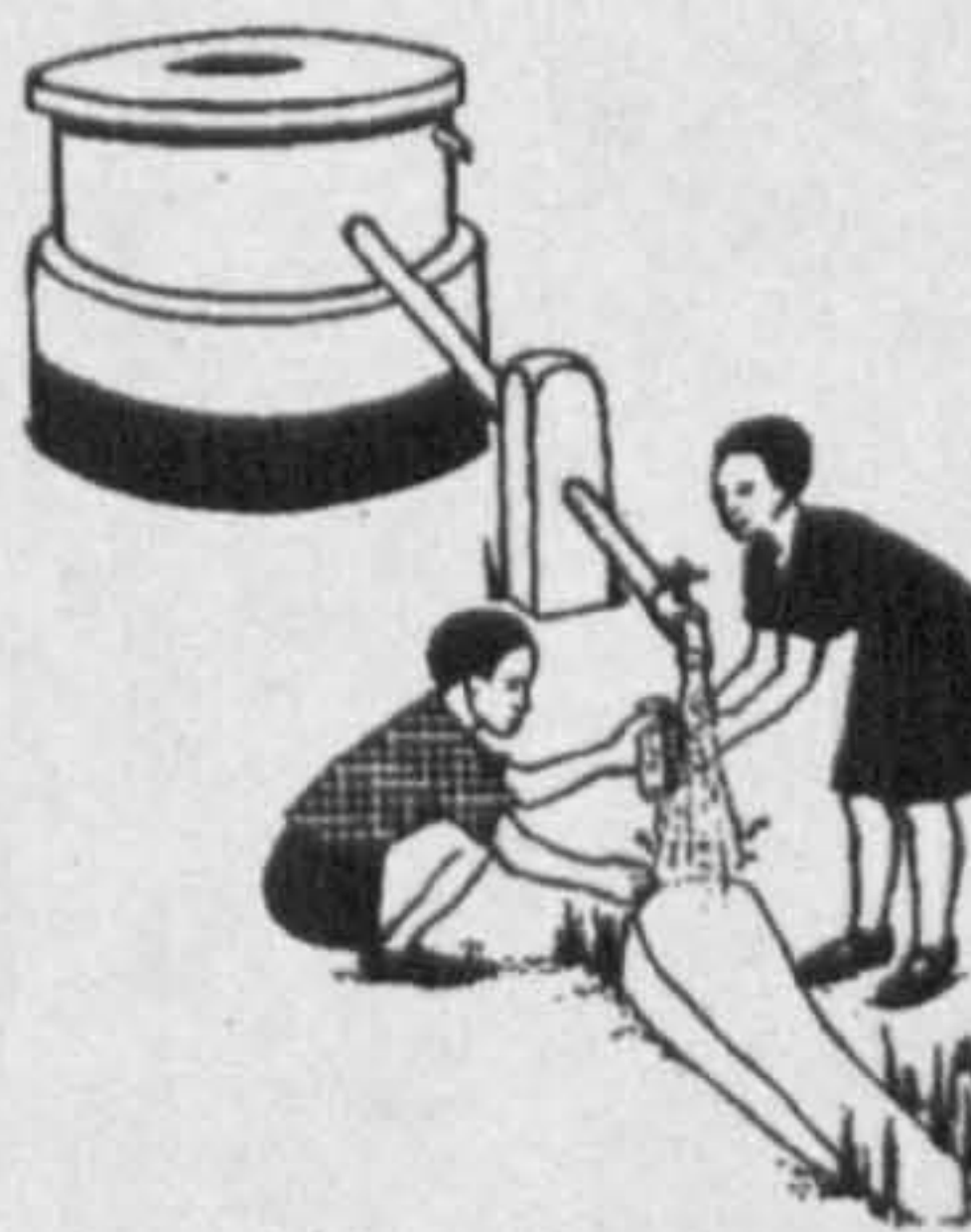
School Sand Filter Tank
