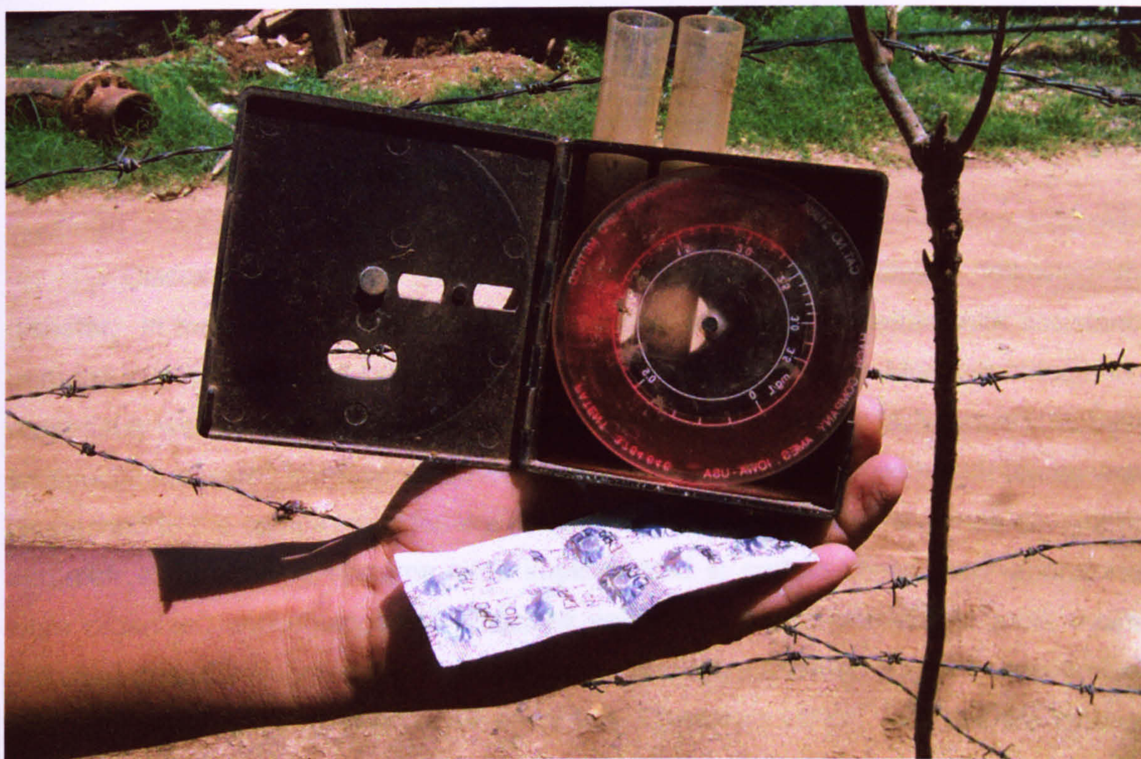
Figure 9.5: Chloroscope shown to an investigator, Tiranagama, Sri Lanka
