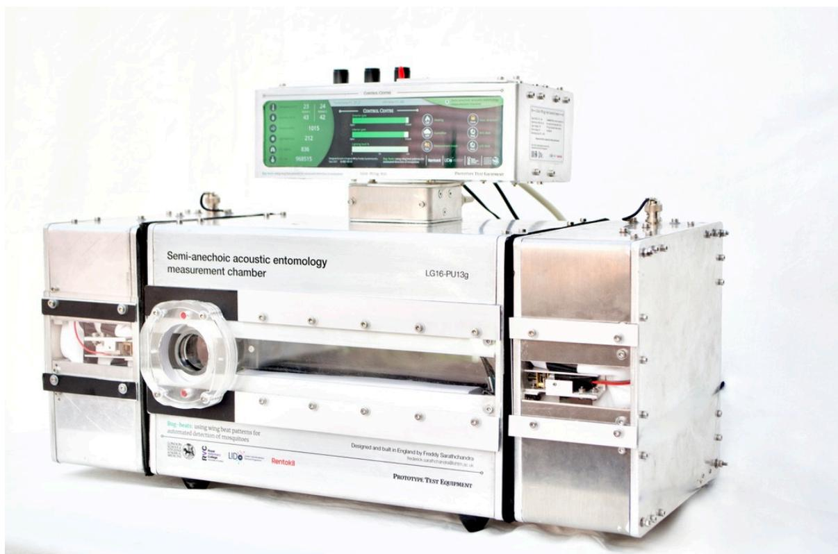
Portable semi-anechoic measurement chamber developed.
