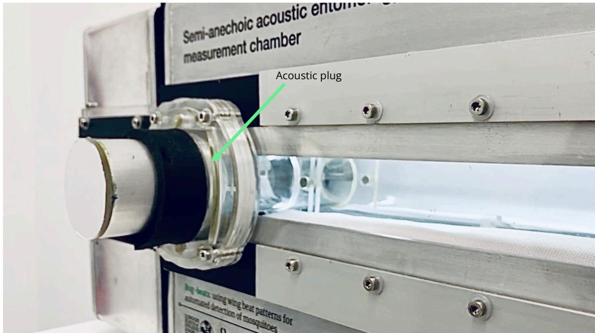
**Figure 3.8** – Exterior view showing acoustic plug in place, secured before opening interior airlock gate
