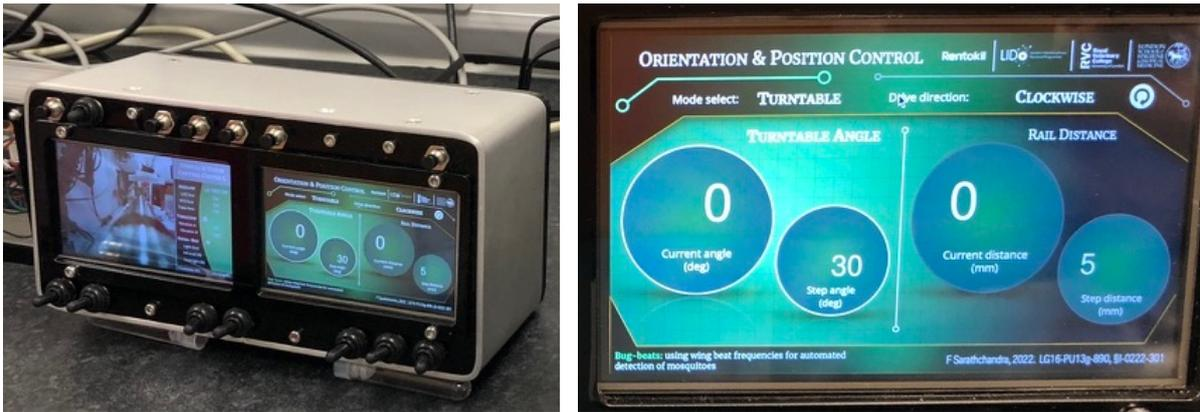
**Figure 3.11a (left), 3.11b (right) – a** , overview of the Position Controller, **b**) detail view of the PU13g-890 user interface for programming the distance and angle
