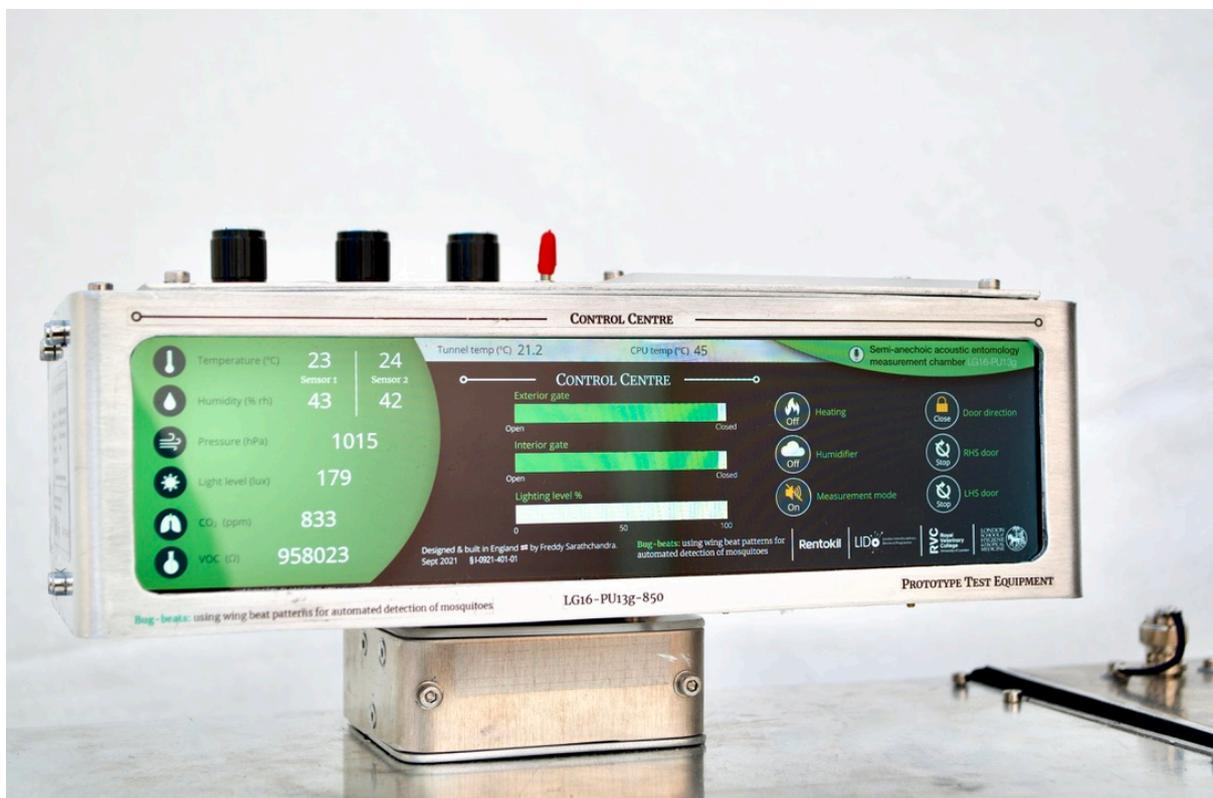
**Figure 3.5** –Control Centre allows monitoring of the chamber environmental sensors and displays status of chamber controls
