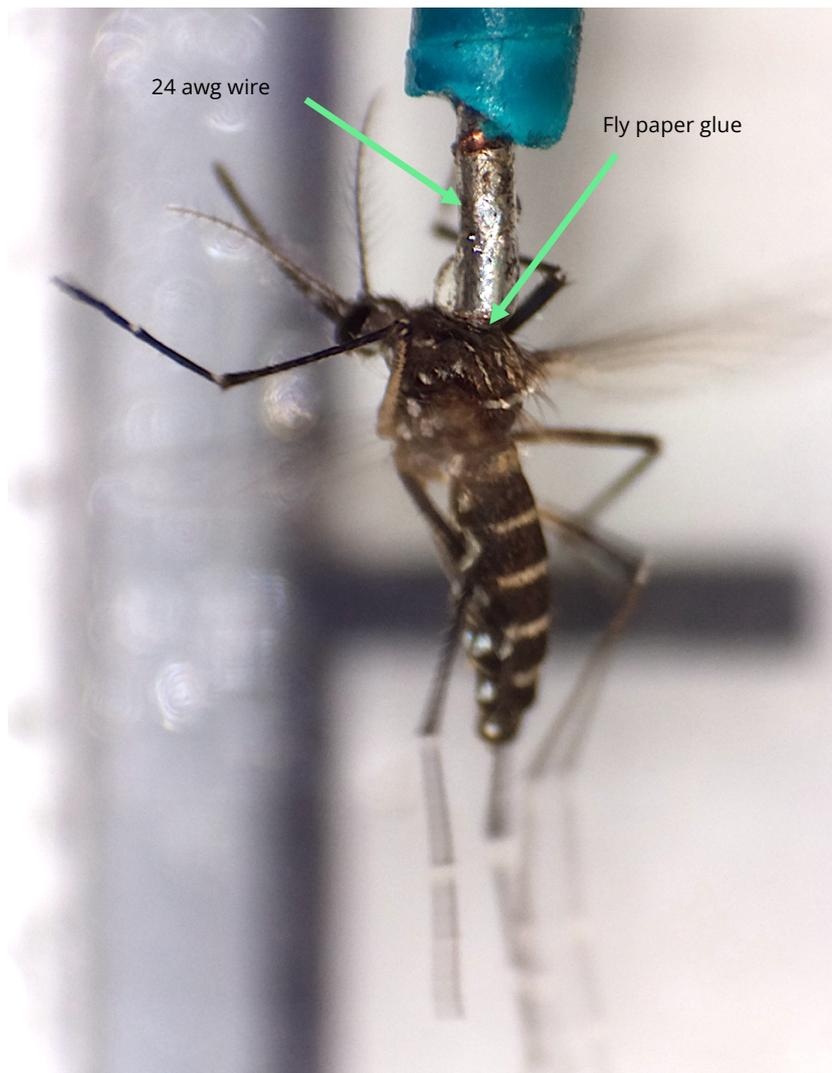
**Figure 3.19** – Detail view of tether position (*Aedes aegypti* female shown)
