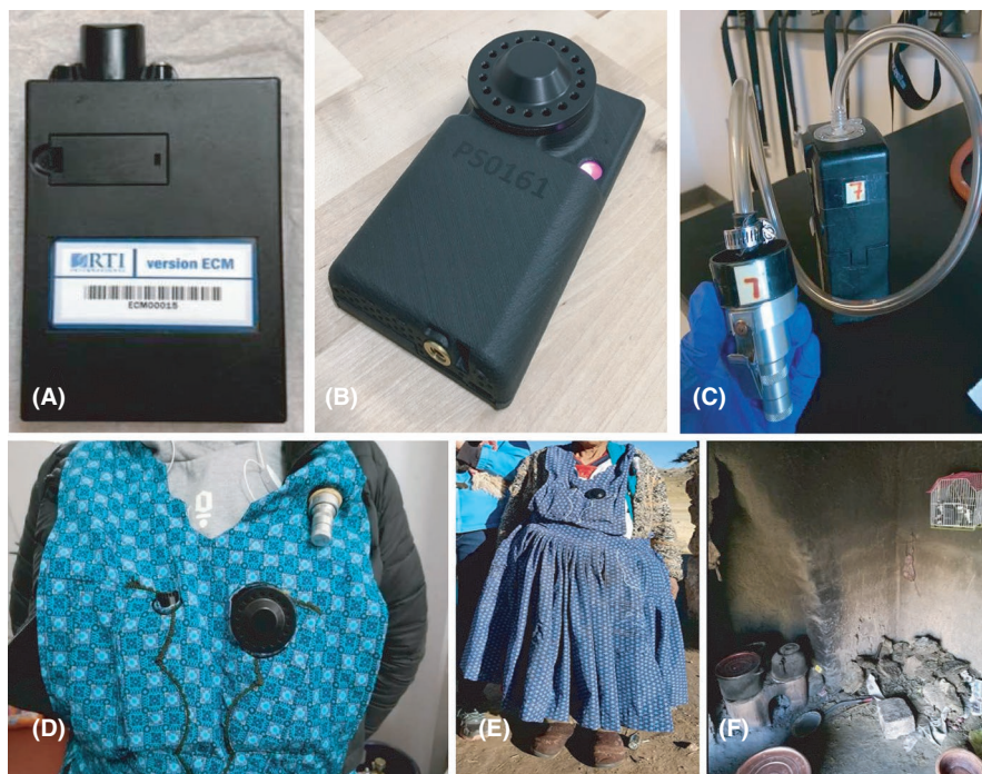
FIGURE 1 (From left to right) – A.) Enhanced Children's MicroPEM (ECM), B.) Ultrasonic Personal Air Sampler (UPAS [photograph from Access Sensor Technologies]), and C.) Triplex Personal Sampling Cyclone with SKC AirChek XR5000 pump [Mesa Labs and SKC]; D.) Shown left to right, the ECM, UPAS, and Cyclone air inlets are co-located on a customized study apron with holes shaped to the instruments; E.) Medium-exposure study participant wearing personalized apron with all three co-located exposure instruments; F.) In-house installation of birdcage containing ECM, UPAS, and Cyclone machines
