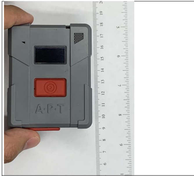
Figure A3. The APT Minima personal air sampler. The monitor is 7.6 cm x 7 cm x 3.2 cm (L x W x H) and weights 138.9 g.
