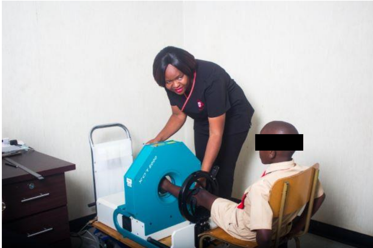
Figure 2.3: An image showing a participant positioned for tibia pQCT scan in the IMVASK study
