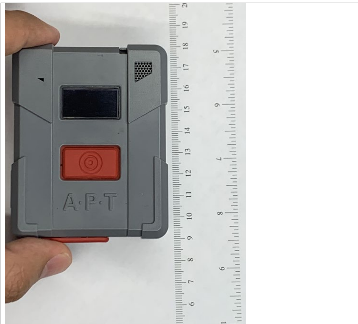
Figure A.2 The APT Minima personal air sampler. The monitor is 3" x 2.75" x 1.25" (L x W x H) and weights 4.9 oz.
