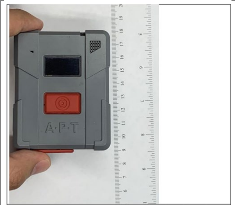
Figure A3. The APT Minima personal air sampler. The monitor is 7.6cm x 7cm x 3.2cm (L x W x H) and weights 138.9g.
