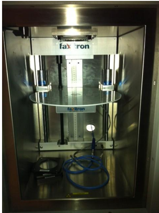
Figure 1: MultiRad 225 irradiation chamber (Cross-sectional schematic reprinted from the Advanced Users' Manual for the Faxitron MultiRad, http://www.faxitron.com/life-sciences-ndt/products/multirad.html ).
