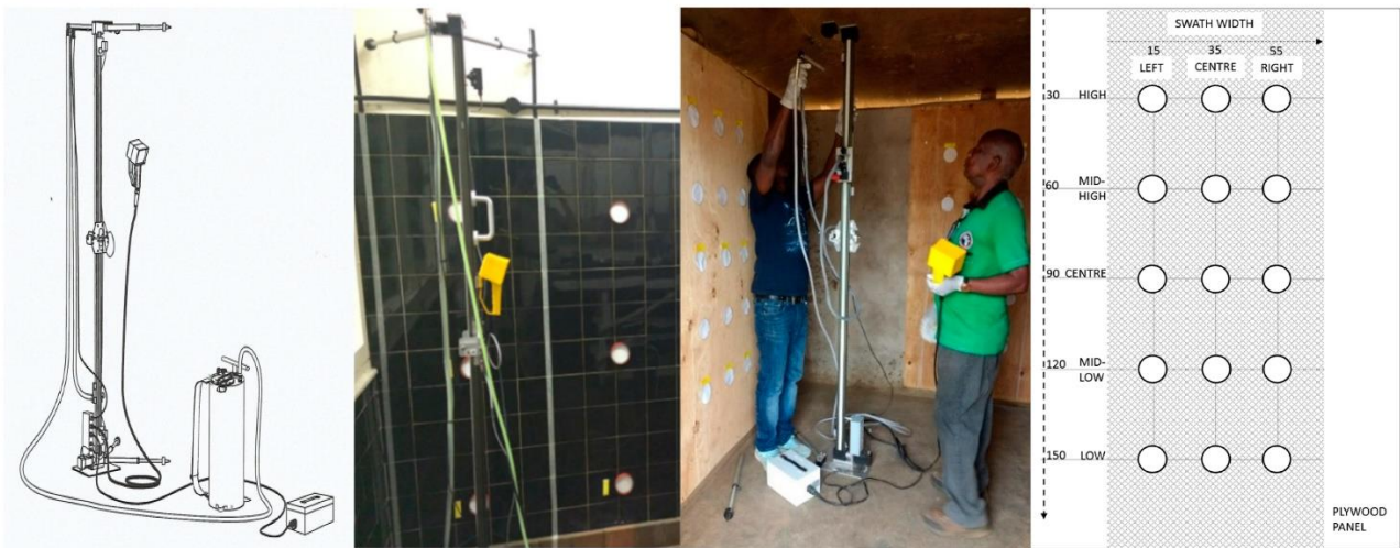
Figure 1. A schematic overview of the sprayer adapted from the Micron product manual is shown on the (left). A photo showing the set-up of track sprayer in the lab (centre left) and in an experimental hut (centre right) is shown, and a schematic overview of the filter paper positions on plywood panels, with values in centimetres, is shown on the (right).
