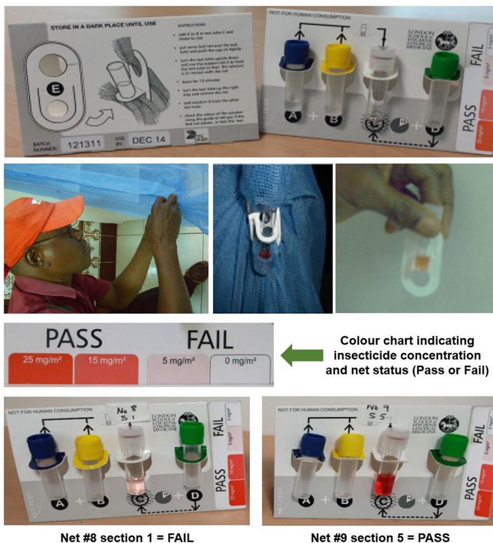
Fig. 3 Colorimetric Test Kit in use attached to the net on Bioko Island to test the insecticide residue of LLINs in situ
