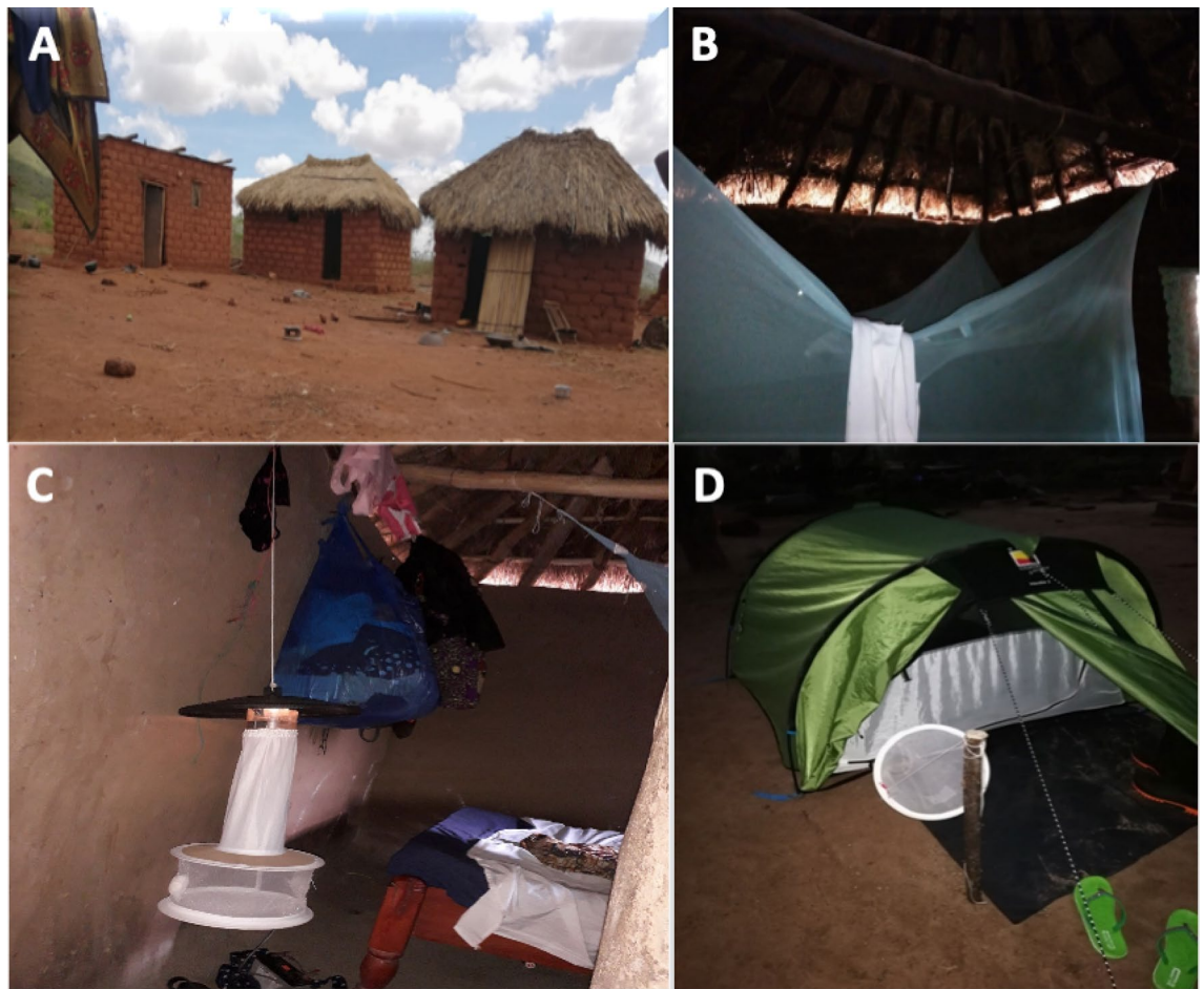
Figure 3. (A) Examples of different traditional house constructions, using local materials. (B) The inside of a typical house with open eaves. (C) A CDC-LT hung at the base of a sleeping space for sampling mosquitoes indoors. (D) A Furvela tent trap set up for catching host-seeking female Anopheles mosquitoes outdoors.
