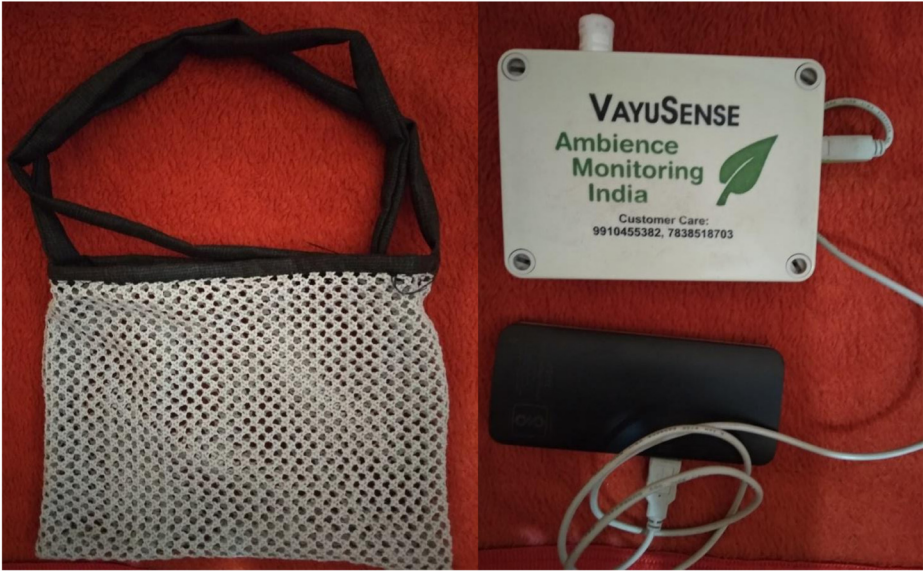
Figure 4. Complete set of device holding power bank and ventilated sling bag.
