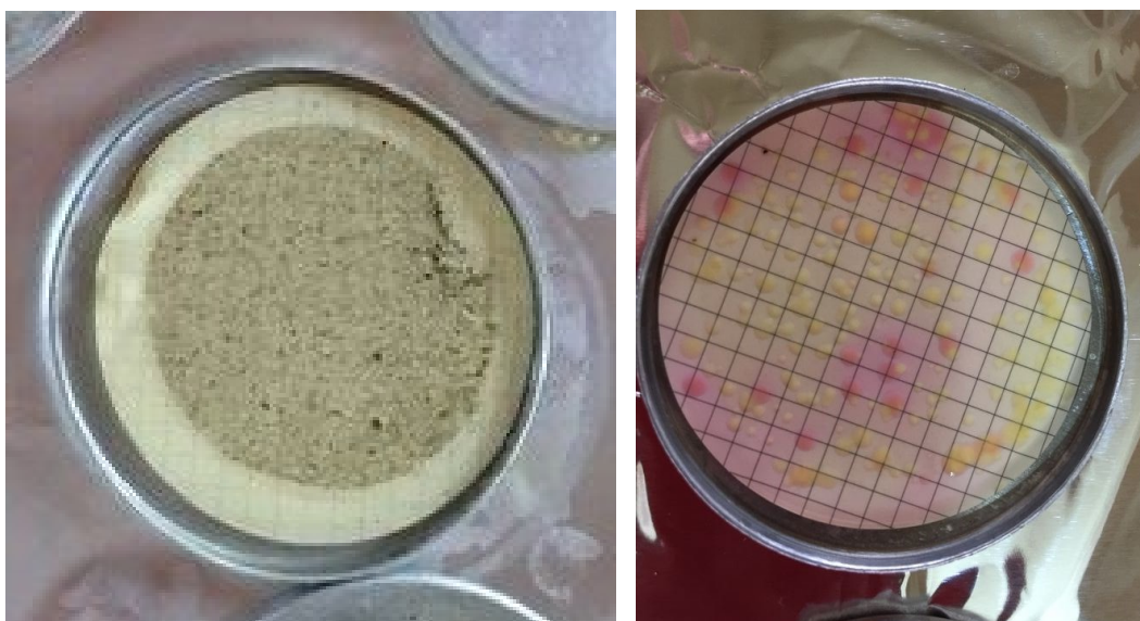
Figure 2-14 Aluminium petri dishes after incubation on lauryl sulphate medium: membrane clogging preventing bacterial growth (left); thermotolerant colonies are colored in yellow (right)
