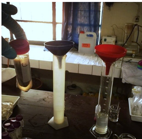
Figure 2-17 Set-up for sample filtration through gauze and APW tube with gauze (left)
