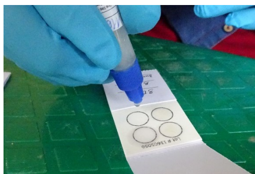
Figure 3-4 Preservation on Whatman® FTA® Elute cards of patient stool, sampled with a rectal swab and eluted in physiological water
