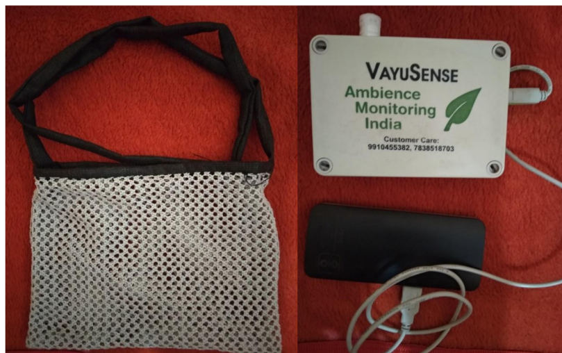
Figure 4. Personal air quality monitoring device with holding power bank and ventilated sling bag.
