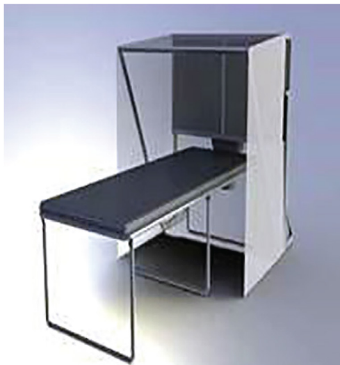
Figure 1 Ventilating headboard. The ventilating headboard consists of lightweight, sturdy and adjustable aluminium framing with a retractable plastic canopy. It is fitted with a high-efficiency particulate air fan/filter unit for filtration (adapted from Mead 48 ).
