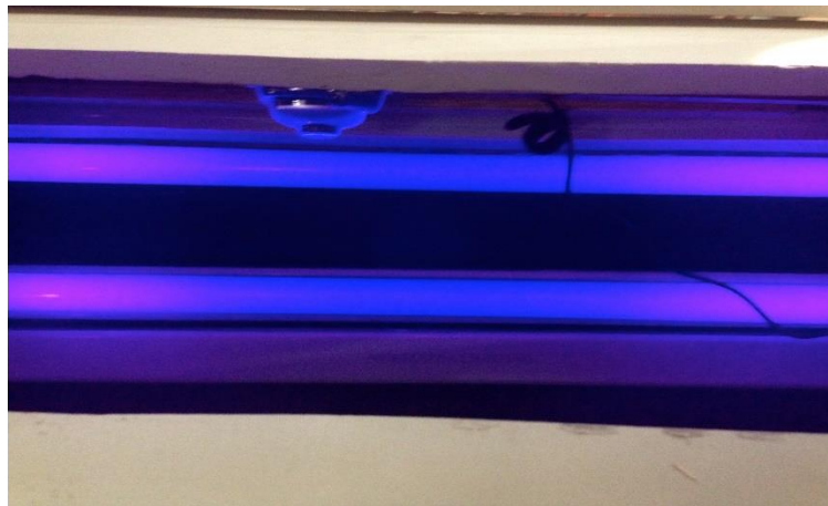
Picture 7.11: Webcam and UV lights installed inside the black box
