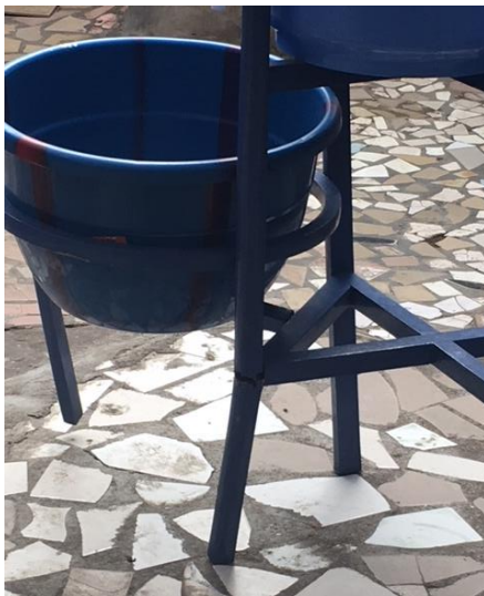
Picture 12.8: HWS with a broken stand (1)
