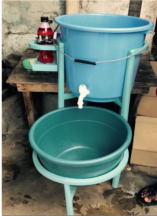
Picture 7.1: Handwashing station's finished product (top bucket's cover removed)
