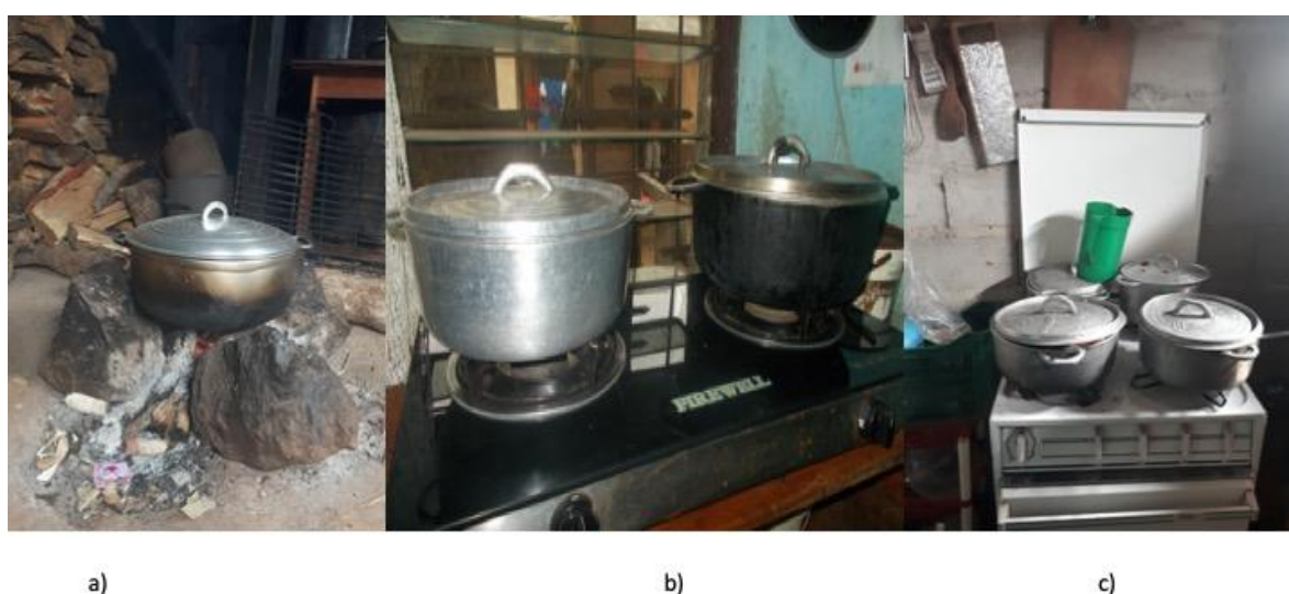
Figure 1. (a) A three-stone fire, (b) a two-burner Liquid Petroleum Gas (LPG) stove and (c) a four-burner LPG stove in South-West Cameroon. Source: LACE Studies.
