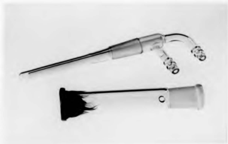
Figure 2.2. Membrane feeding unit with chick skin membrane
