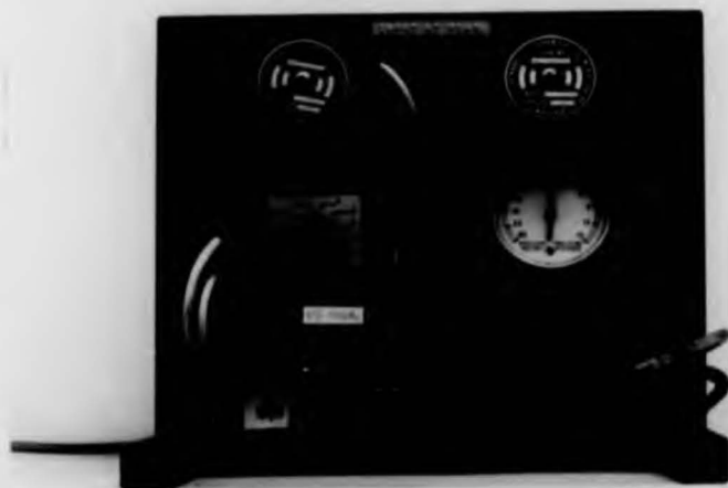
Figure 2.7. Inoculation apparatus, pressure gauge, and timer
