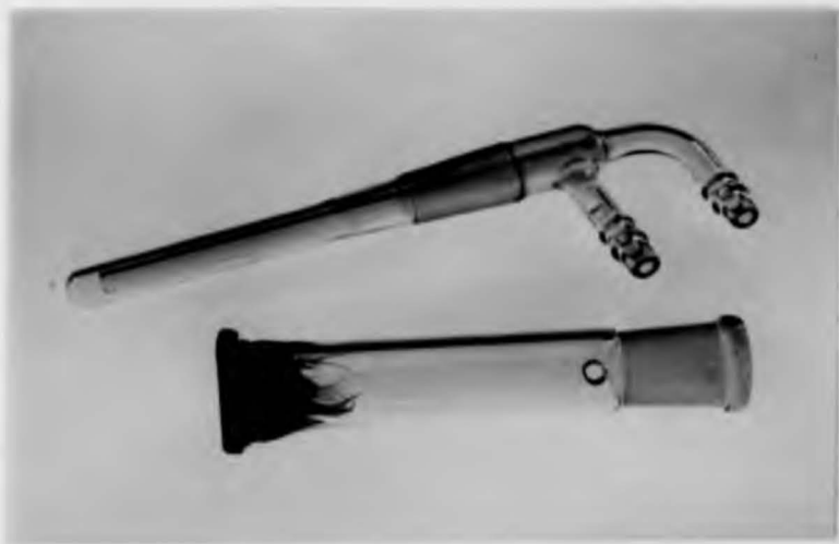
Figure 2.2. Membrane feeding unit with chick skin membrane
