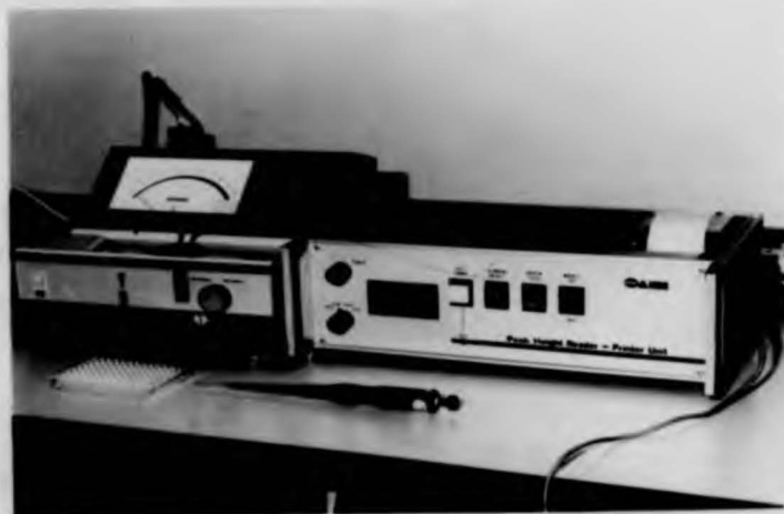
A spectrophotometer (Vitatron, UPM) and printer (Peak Height Reader-Printer Unit, MSE), used for reading and printing ELISA results
