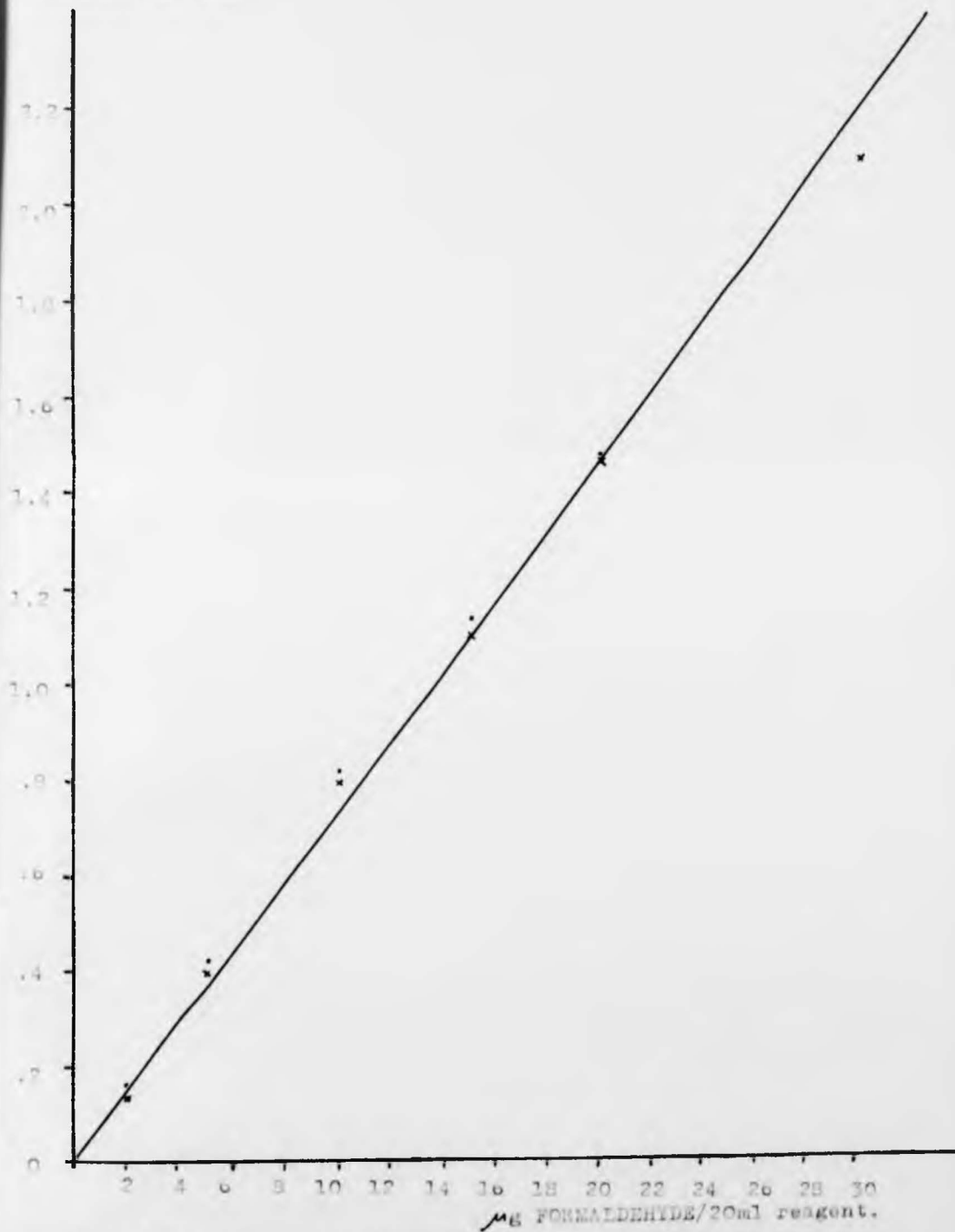
Fig. 2.13. Spectrophotometer calibration chart.
