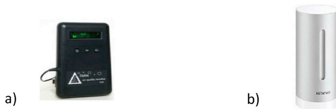
Fig. 2. The a) Dyllos and b) Netatmo sensors used to monitor indoor \text{PM}_{2.5} and noise, respectively.
