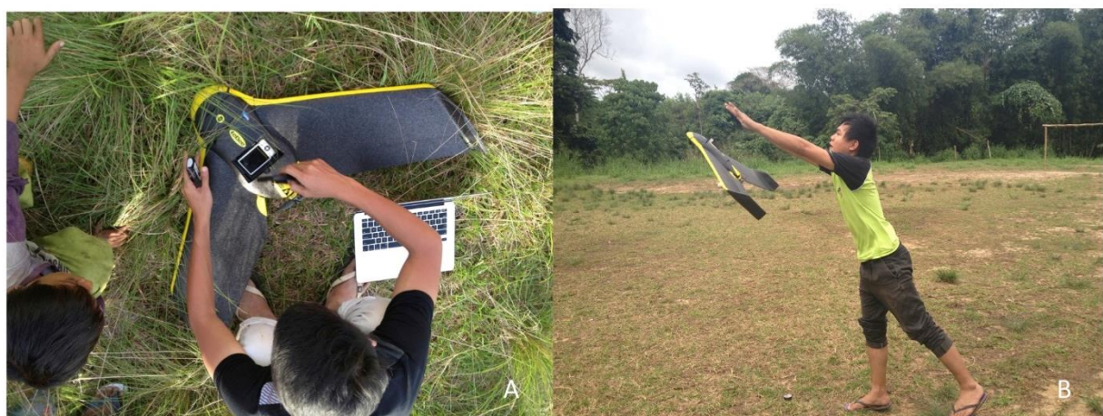
Figure 4.1. Use of the Sensefly eBee to map land cover in Malaysia. A) Setting up the Sensefly eBee before a flight B) Launching the Sensefly eBee
