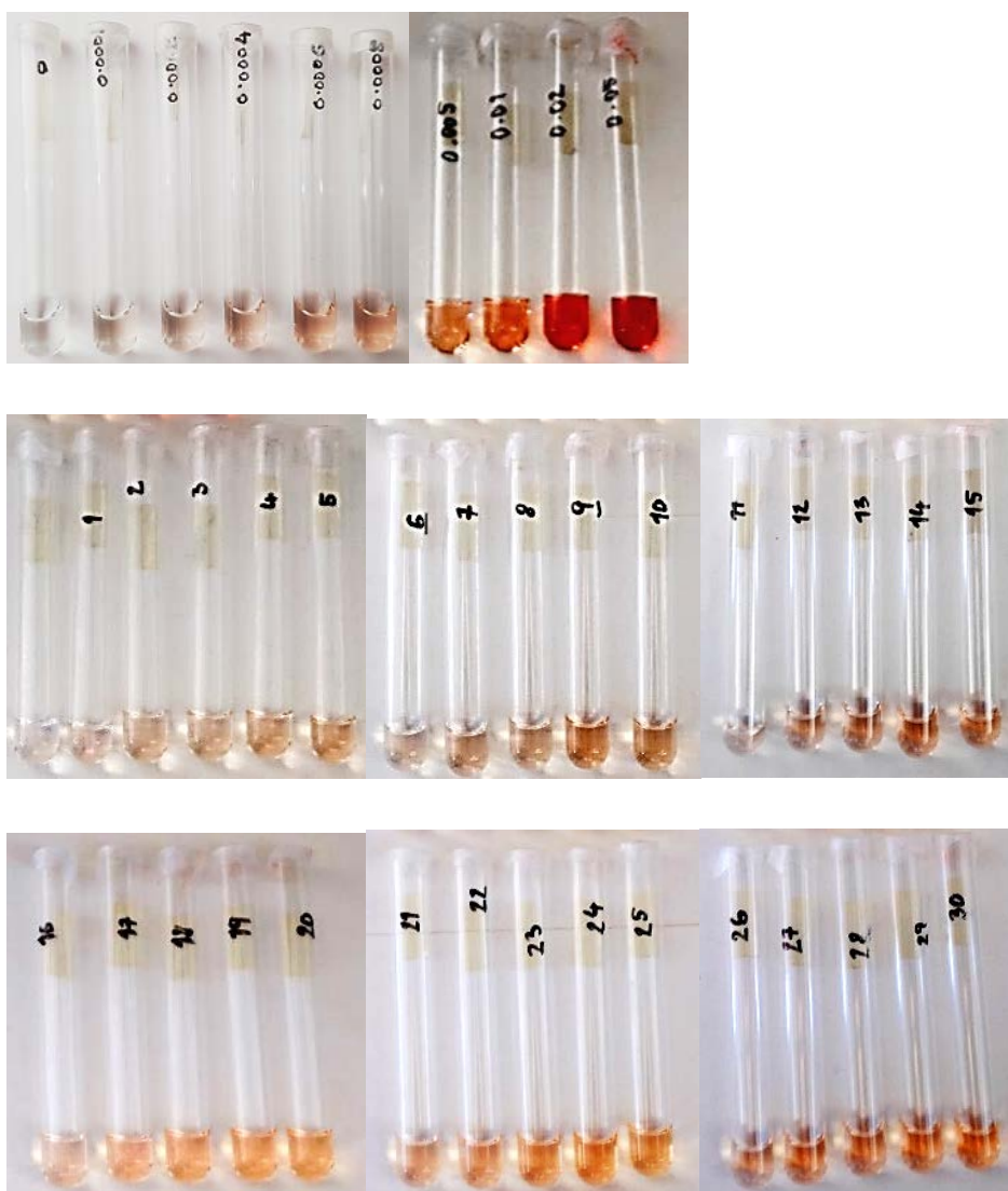
Fig. 3-2. Results of the rapid colorimetric test. Top row left to right: deltamethrin standards at concentrations 0 (control), 0.0001, 0.0002, 0.0004, 0.0006, 0.0008, 0.005, 0.01, 0.02, 0.05 mg/ml. Second row left to right: control; samples 1-5 (0.5 min exposure), 6-10 (1 min exposure), 10-15 (1.5 min exposure). Bottom row left to right: samples 16-20 (2 min exposure), 21-25 (2.5 min exposure), 26-30 (3 min exposure).
