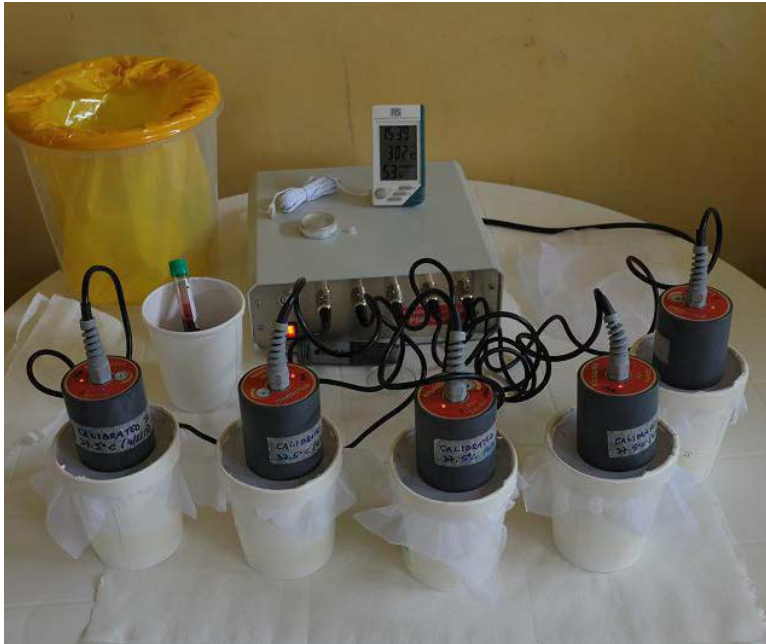
Fig. 2-5. Hemotek membrane feeding system was used in direct membrane feeding experiments. Feeders were held at 37.5°C throughout the feed. Parafilm artificial membrane was used.
