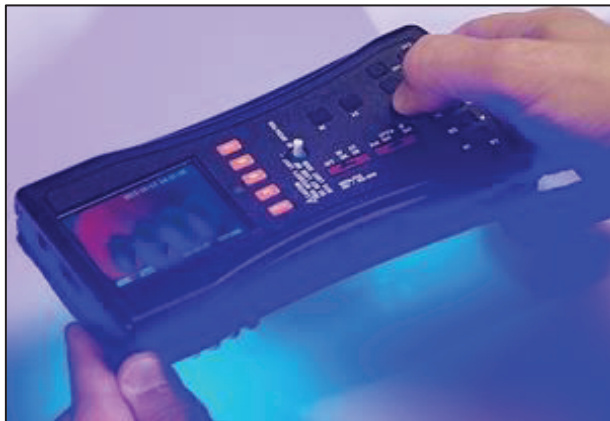
Figure B4: The Counterfeit Detection Device (CD3+) Source: from United States Food and Drug Authority website.
