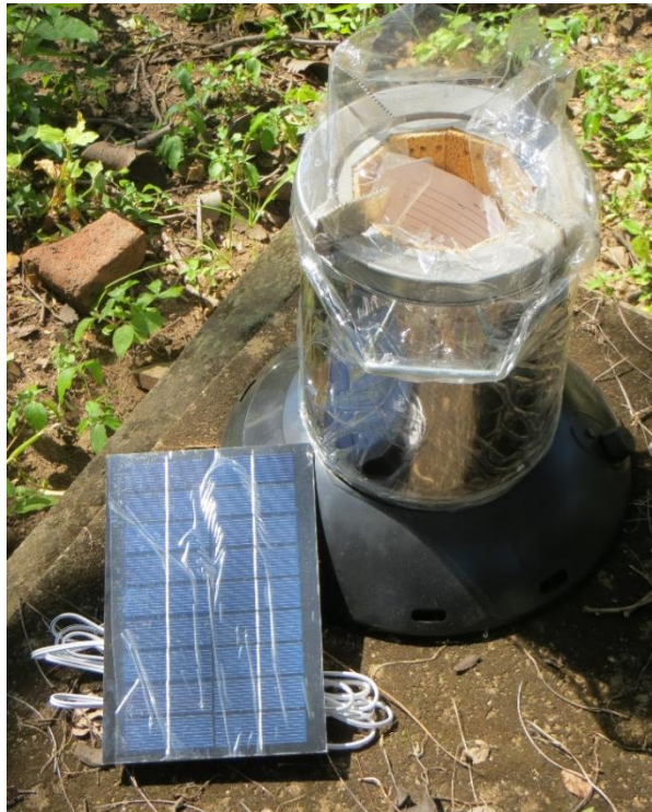
Figure 3.4 Philips fan-assisted cookstove and solar panel
