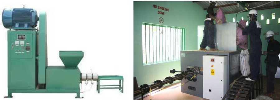
From left: example of Screw-Press Biomass Briquette Machine, Mechanical Biomass Briquette Machine in The Gambia
