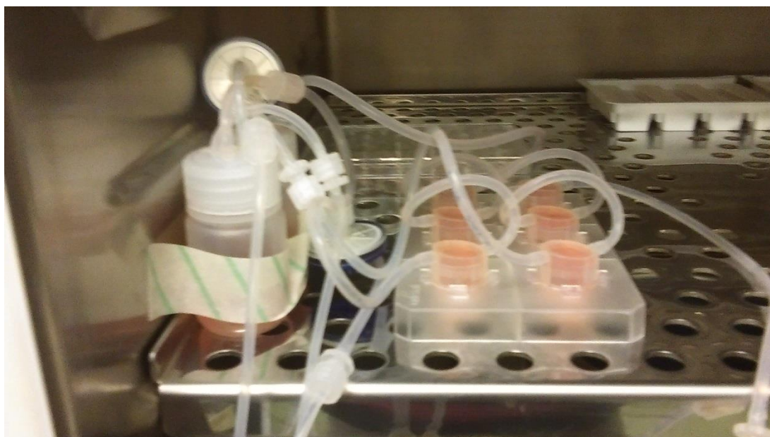
Figure 2.3-3. Photograph of the QV900 media perfusion system
