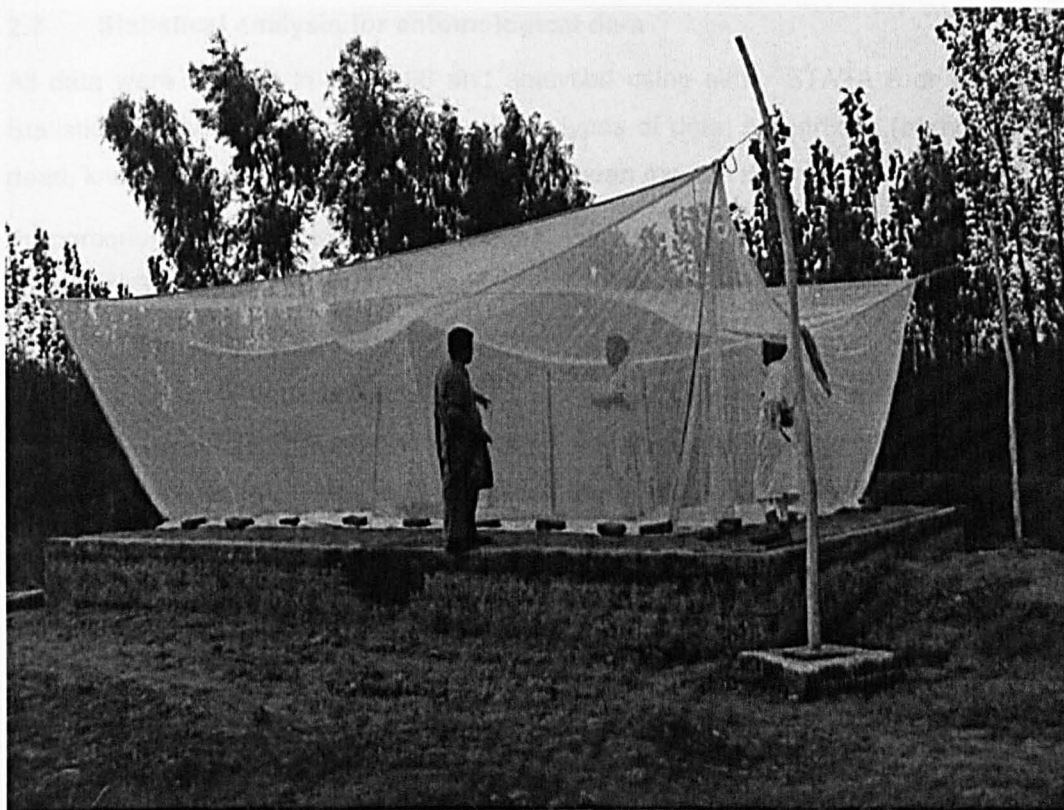
Figure 2-1. Overnight outdoor platform, test materials in readiness for a nights testing.
