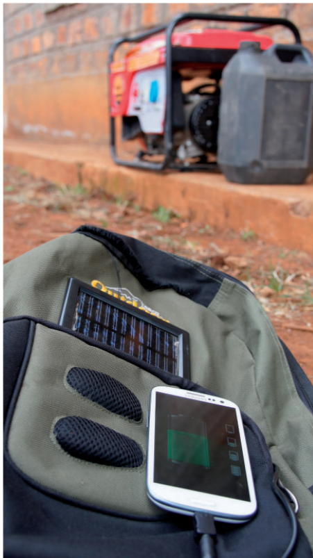
Figure 3. A solar-powered rucksack as used by the Peek healthcare workers visiting patients door to door, negating the need for a mains power supply
