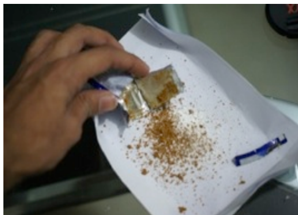
Right: Pureit sachet in Pakistan, visibly humid, discoloured and sticking to the sachet inside Left: Seams where perforations were most likely (courtesy C.Dorea)
