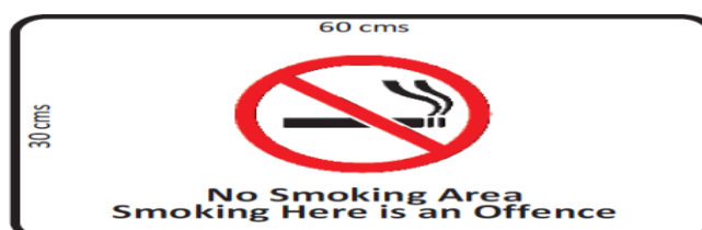
Figure 5.1: Specifications of the 'no smoking' board to be displayed at conspicuous locations at all public places in India
