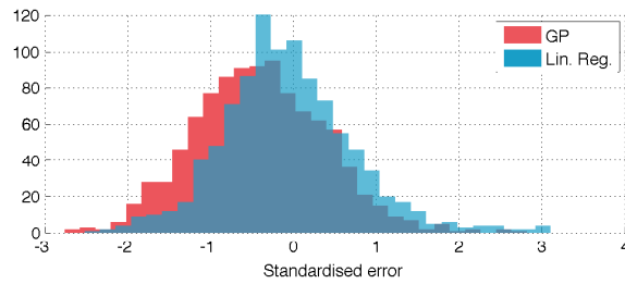
FIG. 6. Standardised errors for the GP and linear regression based emulators for predictions of the wave 8 simulator runs. Most errors lie within the [-2, 2] interval. The GP emulator's errors have a slight negative bias, and the linear regression emulator errors are slightly skewed towards positive values.
