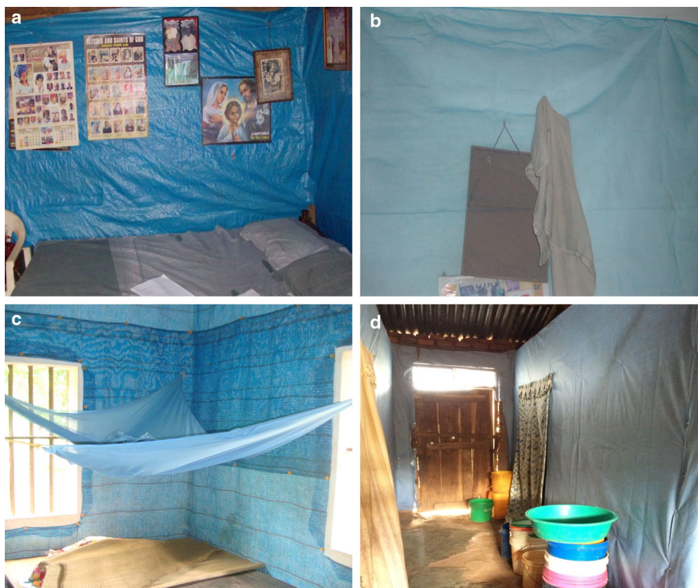
Fig. 1 Commercial ITWL products. a Polyethylene plastic sheeting (ZeroFly®). b Polyester netting (PermaNet® 2.0). c Polyethylene woven shade cloth (ZeroVector®). d Polypropylene non-woven fabric (PermaNet® Lining)
