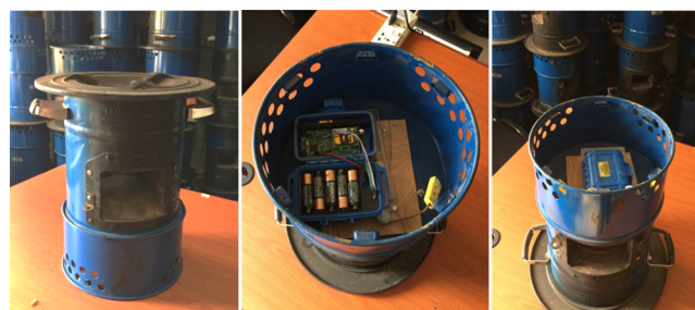
Figure 1. Temperature sensor installed within improved cookstove false-bottom. A metal cover encloses the false-bottom and obscures the sensor from view.
