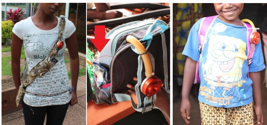
Figure 1 Personal exposure monitoring equipment set-up for cook and child under 5. Left : Main cook air monitoring set-up as worn. Top to bottom: HOBO Pendant Temperature and Light Data Logger; HPEM; GasBadge Pro; TuffPro Pump. Centre: Child HAP monitoring backpack with HPEM, tubing, and arrow pointing to fabric-covered GasBadge Pro. Right: Child air monitoring set-up as worn.
