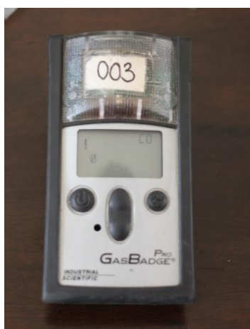
Figure 2 GasBadge Pro for measuring carbon monoxide (CO).
