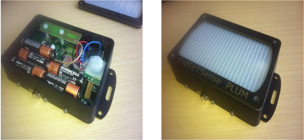
Figure 5-14: The first version of the SweetSense PLUM (June 2012) – the internal fitting and the encasing
