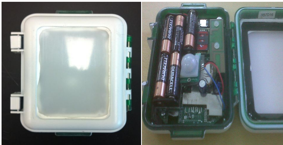
Figure 5-6: The SweetSense (SS) PLUM - an external and internal view of the final version used in the study
