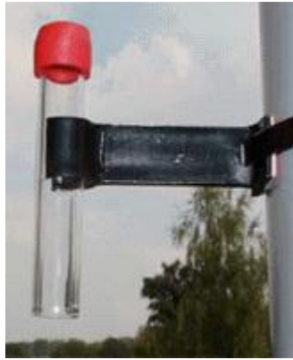
Figure 10: A Palmes Diffusion Tube (Presentation slide from WHAP project meeting June 2013).
