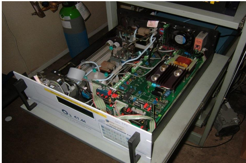
Figure 3: Inside an air pollution monitor (Personal photo).
