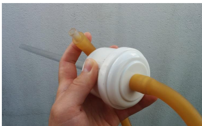
Figure 3.1: Manual aspirator used for human landing catch collections, model 612 (John W Hock).
