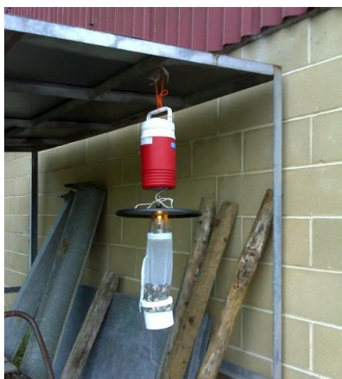
Figure 2.1: A CDC light trap baited with CO 2 provided by ~2kg of dry ice in an igloo, in situ next to the cattle sheds at Coombelands Farm.
