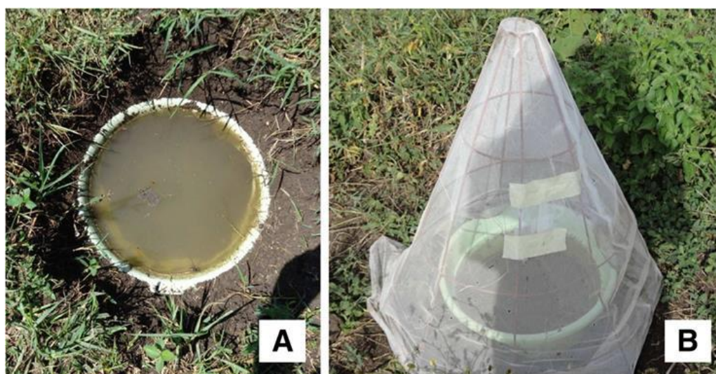
Figure 3.1: Set-up of standardized field test. (A) Enamel-coated bowl sunk into the ground and filled with water and soil to simulate a natural pond. (B) Netting-covered emergence trap on top of a pond to prevent escape of emerged adults.
