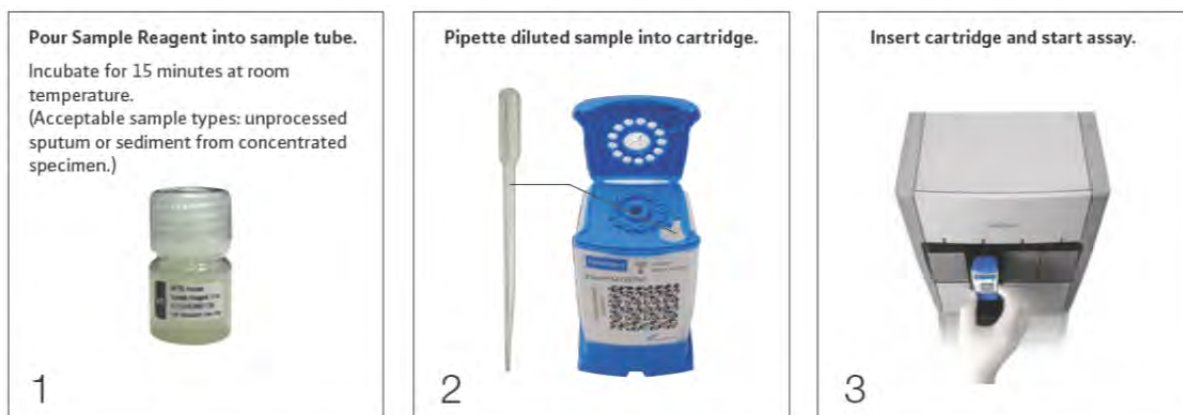
Figure A-3 Manual steps for sample preparation
