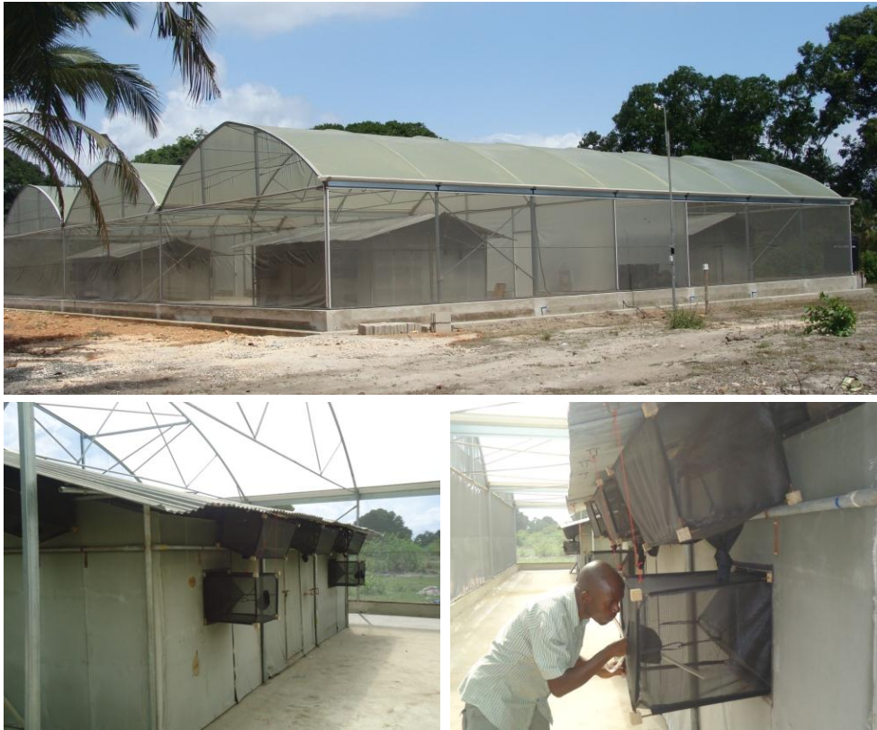
Figure 4.2. Semi-field system. The walls and the roof of the semi-field system (SFS) are made of metal frames and fibreglass netting material. It was divided into four equal square sections divided by fibreglass netting. An experimental hut was placed in each compartment. The SFS [14] allowed replication of experiments within a short period of time. Laboratory reared mosquitoes were used and were available throughout the duration of experiments hence there were no delays as usually experienced in the field.
