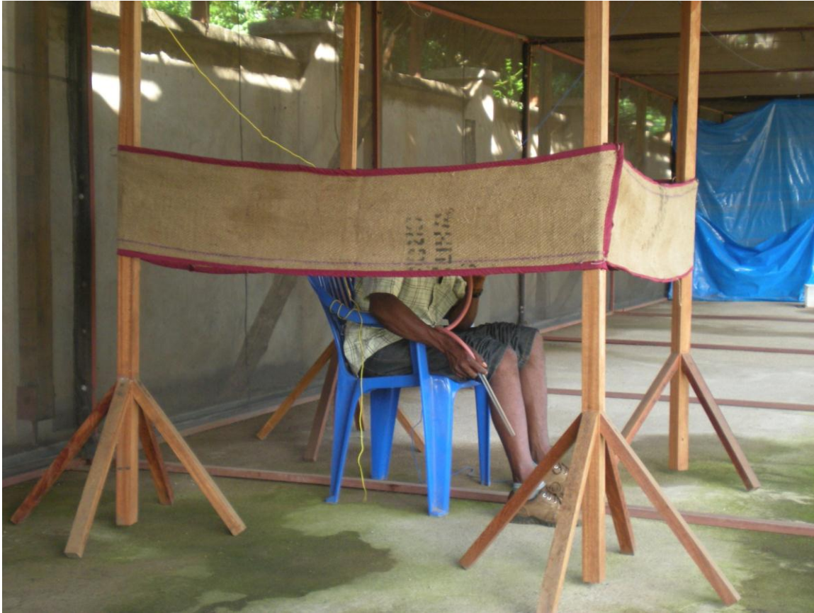
Figure 6.1: Transfluthrin hessian strip. The hessian strip is made from fine sisal fibre woven together to make sacking fabric. The strip is 4 \times 0.3 m long. It is treated with transfluthrin. The strip is suspended on 4 wooden poles making approximately 1 \text{ m}^2 area surrounding the human participant conducting mosquito catches.
