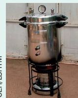
Figure 1: Diagram of a kerosene-burning steam-pressure autoclave
