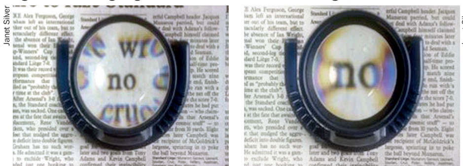
Figure 4. Increasing magnification reduces the field of view (right)
