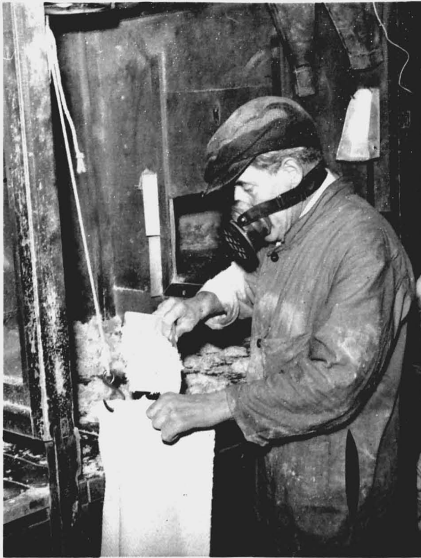
(3) Filling the mattresses with amosite asbestos fibres.
