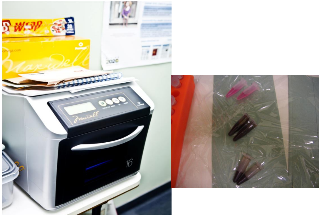
Figure 4k: DNA extraction machine (Maxwell™ Automated Purification System, Promega, USA). Whole blood mixed with Trizol reagent (Invitrogen, UK) for RNA extraction
